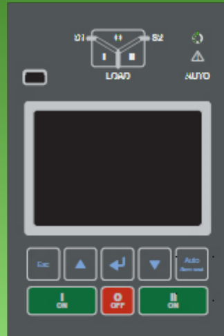
Door Mounted, Lockable Cover, Type 3 Controller Standard
